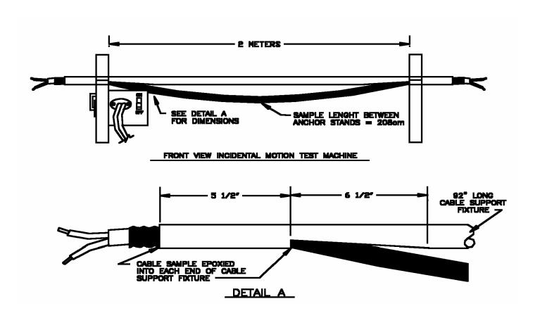
Figure A.1—Front view with cable support detail
