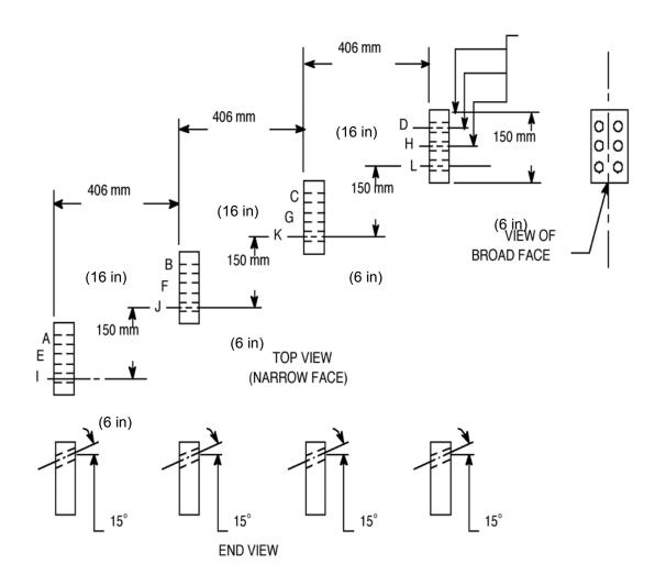
Figure 1—Test setup for pull-through metal plates test
