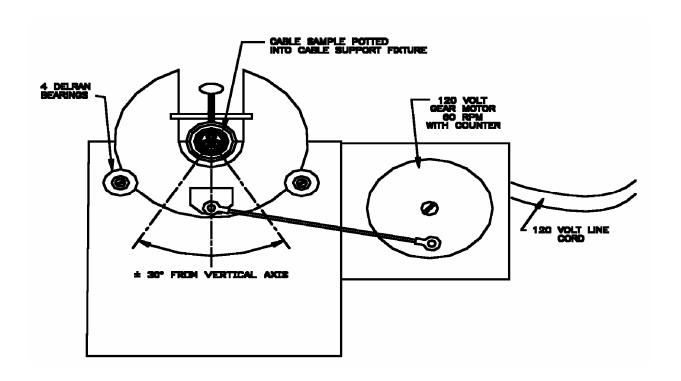
Figure A.2—Motion mechanism detail
