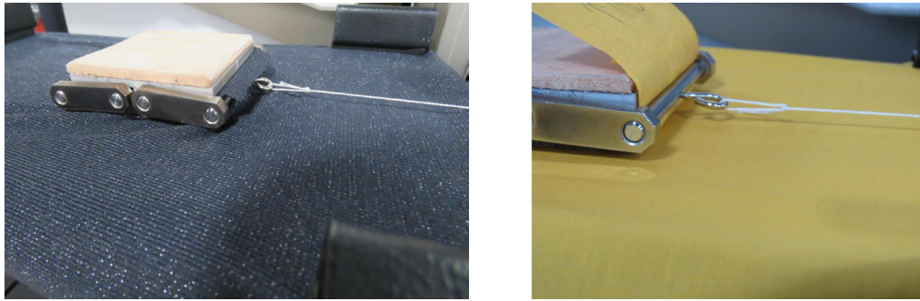
FIGURE 22: A LOW TENSION HAS BEEN APPLIED TO AVOID BUCKLING DURING THE MEASUREMENT
