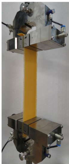
FIGURE 18: (A) CYCLIC TENSILE MEASUREMENT BY ZWICKROELL, (B) OBTAINED STRAIN-STRESS CURVES
